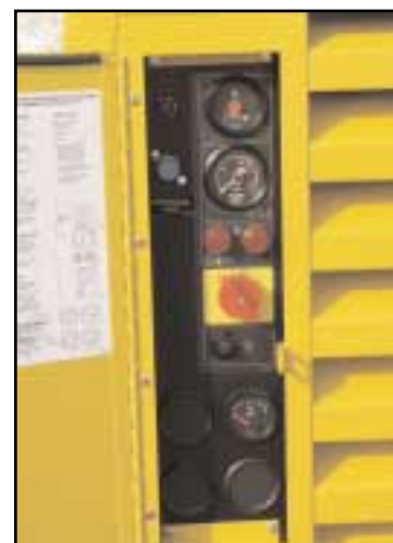
Instrument Panel – All necessary push buttons and gauges are grouped on a single panel for easy monitoring.
